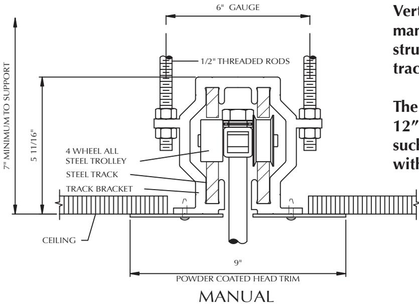
Vertical steel track is to be used only for curved walls, manual or electric. Smooth operation and rigid construction allows the designer freedom to make the track system fit the building.
